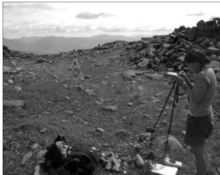
Val Stori entering data into a GPS unit. The camera on the tripod has a fixed focal length and is set up over a small pin fixed in a rock.
